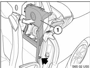
25. Carefully unclip lower Left panel (indicated by black arrow), then remove Left panel (1) from vehicle.
