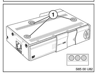
2. Cover the holes where the shipping screws were installed with the 3 adhesive seals (1) supplied with the unit.
