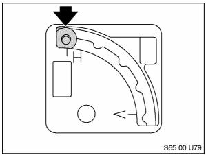
3. Adjust the CD changer mechanism pins for proper settings. Mechanism should be set to "H" on both sides of unit for horizontal mounting position.
