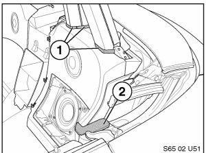
21. Remove rubber strips (1) around both left roll bars. Remove rubber cap (2).
