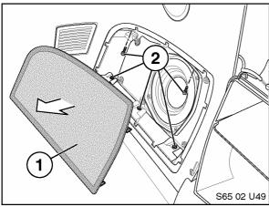
19. Remove Right Speaker Grille (1) by carefully pushing outwards (from the rear) or with a non-marring pry tool. Remove 5 T20 Torx screws from Right panel (2).
