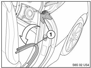
24. Pull back drivers door weather-stripping (1) to expose edge of Left panel.
