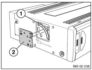
4. Affix the locking squares (2) on the left and right sides of the CD changer chassis to firmly secure the pins (1) in place.
