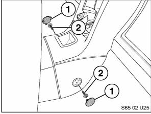
7. Slide seats forward. Remove left and right lower panel covers (1) and mounting screws (2).
