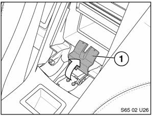
8. Lift rearward and remove switch panel cover (1) to expose mounting screws.
