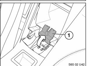
8. Lift rearward and remove Switch Panel Cover (1) to expose mounting screws.
