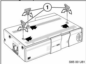
Remove the three shipping transport screws
