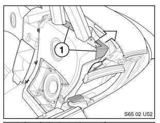
22. Carefully pull rearwards on rear panel cover (1) and remove from vehicle.
