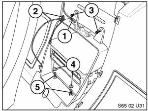
Note: To complete the following steps it will first be necessary to engage the manual release (1) and lift the convertible top (2) from its locked position by at least 3 inches.
