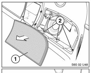
18. Remove Left Speaker Grille (1) by carefully pushing outwards (from the rear) or with a non-marring pry tool. Remove 5 T20 Torx screws from left panel (2).
