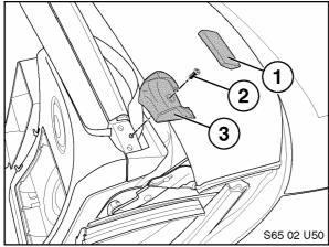
20. Carefully remove Left seatbelt guide cover (1), then remove T20 screw (2) and seatbelt guide (3).
